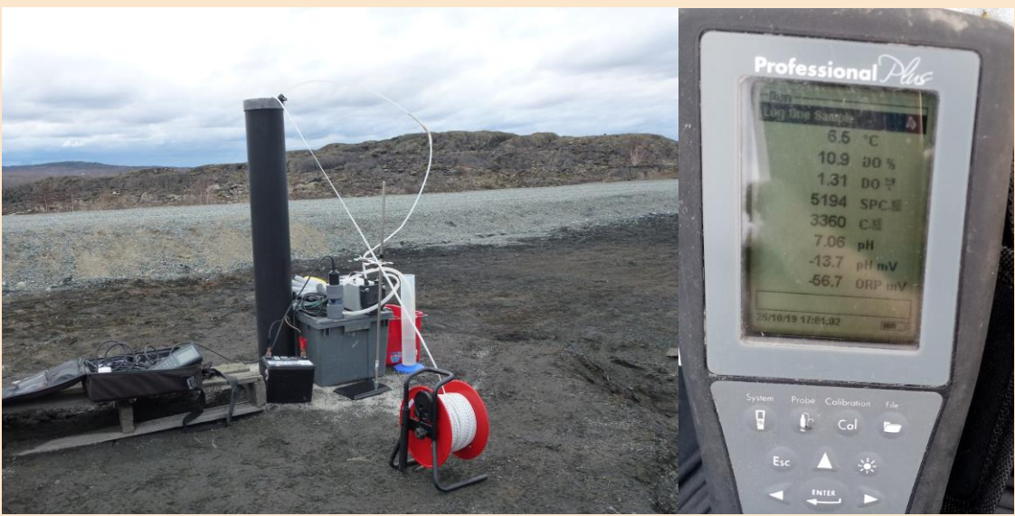
Figure 3 : Low-flow sampling, with monitoring of the physico-chemical parameters of well Q2-R-PO-02-18 on Quémont-2 site
