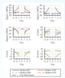
consisting of the three induced stress components and three components are generated to visualize the differences between various scenarios by changing the aspect ratio, dip, strike direction, as well as the geometrical configuration of the modeled plane. Figure to the left as an example is the comparison made to simulate increasing strike direction with respect to the global X-
