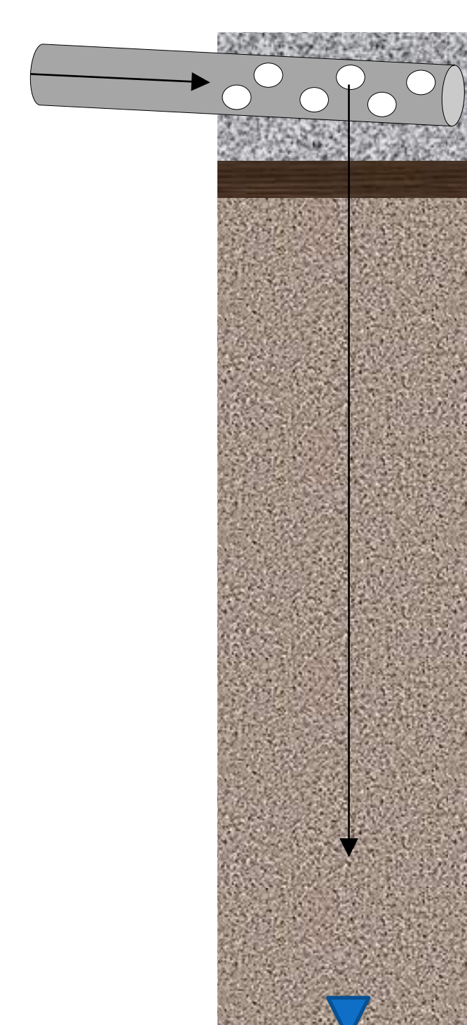
Figure 4: Vertical OWTS filter. Three standard layers used in modelling contaminant transport shown (from top down): the gravel distribution trench, a thin biofilm, and a long sand filter. Arrows indicate septic tank effluent percolation.
